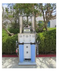
The following units are WALL MOUNTED commercial reverse osmosis units. Frame is constructed of welded Stainless Steel. Width is 36" (brackets 32" on center), out from wall 10" and the height varies from 26" to 44" depending on output. All are fully tested, and have inlet 5 micron and carbon cartridges, low pressure switch, tank fill control, pressure gauges, recirculation pressure set valves, auto adjust drain control. Numerous options available.
